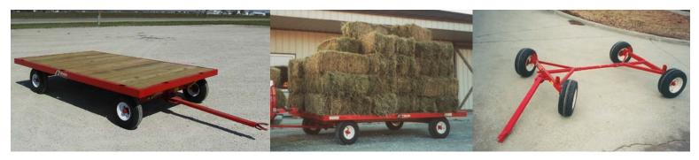
6' x 10' Jr. Flat Rack has 2" treated floor on 3 x 6 sills and is framed all around in steel with stake pockets. Its low 21" deck height makes loading E-Z. It can haul up to 50 bales and is very useful in orchards and nurseries, for landscaping and displays. Narrower widths are also available for vineyards, and factory in plant use.
