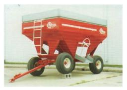
400 Bu. 8-1/2' x 12-1/2' on 1384B 14L x 16.1 tires. Welding shops have inquired about selling 116" our wagons because they weld & repair other brands of wagons but they seldom have to repair an E-Z Trail. The oscillating axles do make a difference.
