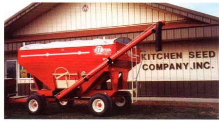
The optional cover has an 18 oz. reinforced vinyl roll tarp, stainless steel end caps, & *Shur-Lok* latch plate to keep seed dry at planting time. You can safely cover or uncover your seed in 30 seconds without climbing on the wagon. Since some "stretch & shrink" is normal, an optional rear ladder is the ideal holder for the roll crank. Proper tarp tension is easy to maintain by simply hooking the crank to a higher or lower ladder rung.
