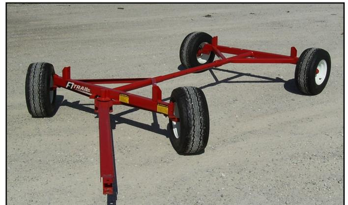
2-Ton Jr. Running Gears are available in 46” or 60” wheel tread & std. 5.70-8 tires (shown here with opt. 20.5 x 8-10 tires). E-Z Trail’s time-tested “wag-resistant” steering utilizes a kingpin with tapered roller bearings & greasable automotive tie rod ends.
