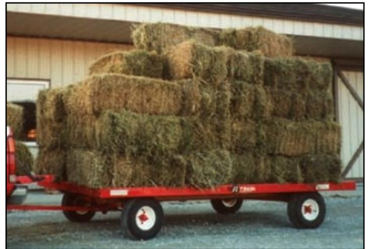
**Jr. Flat Rack:** 6’ x 10’, 2-ton gear with std. 5.70-8 tires or opt. 20.5 x 8 tires, 2” x 8” treated floor boards (40 yr. wood life) framed in steel with stake pockets. Its low 21” deck height makes loading E-Z. It can haul up to 50 bales and is very useful in orchards & nurseries, for landscaping & displays. Custom rack sizes are available for use in factories, vineyards, etc.
