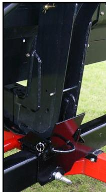
Special brackets are available to fit various models of flex draper heads
