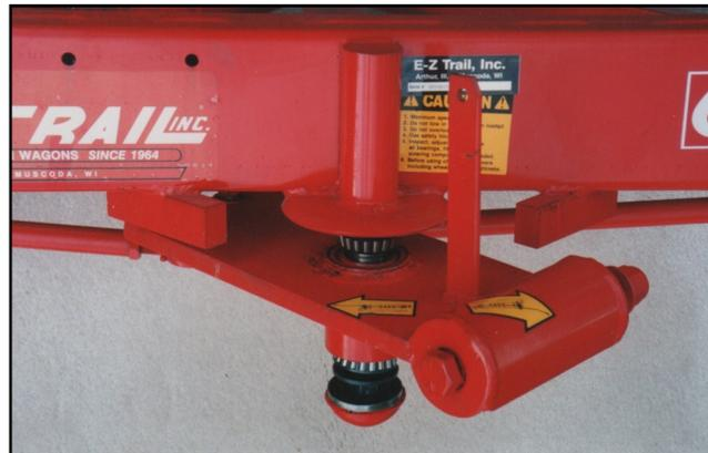
"Lifetime" accurate trailing is assured by E-Z Trail's original steering centered around sealed tapered roller bearings, truck type ball joints and dual stops with 100% greater oversteer protection. All steering parts are weather protected for lifetime outdoor use.
