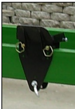
Dual tie-down ratchets are standard.
