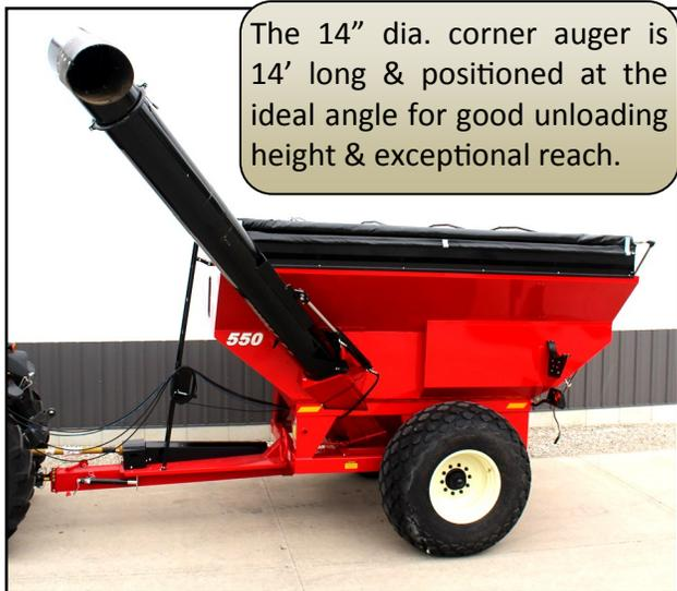
The 14" dia. corner auger is 14' long & positioned at the ideal angle for good unloading height & exceptional reach.
