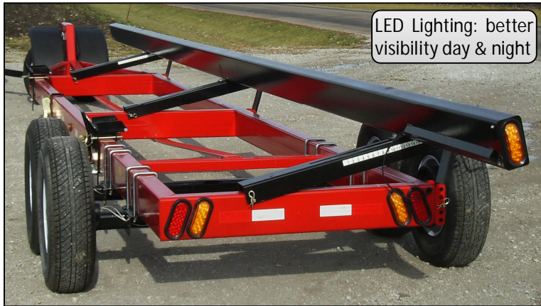
Center pivot equalizes load weight and shock for dolly wheels over dips, bumps & rough terrain
