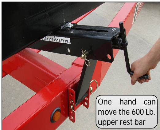
Hook-up time & effort is reduced with the E-Z Lift spring & telescoping tongue
