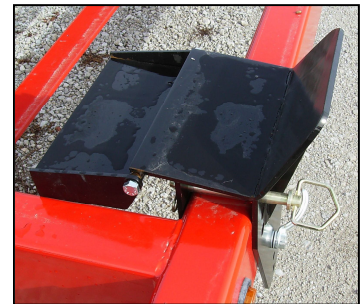
Lower rest: the two-way slider bracket easily accommodates a wide range of header styles without needing special brackets
