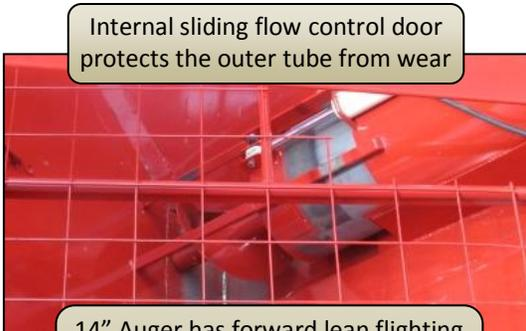
Internal sliding flow control door protects the outer tube from wear
