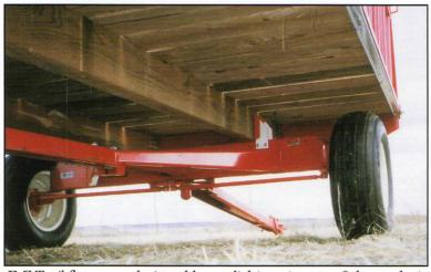
E-Z Trail floors are designed lower, lighter, stronger, & longer lasting. The 2 x 8 floor boards and 4 x 8 sills are made of Southern Yellow Pine treated for long life. The special cut sills are 27% stronger than commonly used 6 x 6 sills, according the the University of Wisconsin Forestry Dept. The floor is framed all around in steel for added strength and warp prevention. Since there are fewer collection points for residues which cause wood decay, floors will stay cleaner and last longer.
