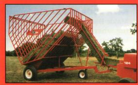
Bale Baskets are also available: By harnessing energy that's absolutely free, one man can bale up to 10 bales per minute without a bale thrower. Compressed energy released from the baler simply pushes bales up the chute. Hundreds of satisfied customers are saving crucial time and labor.
