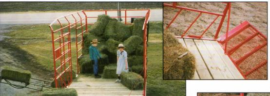
The front gate & side doors are mounted flush to the floor & made of flattened expanded metal which provides a smooth "slide" exit for unloading heavy bales **without** lifting.
