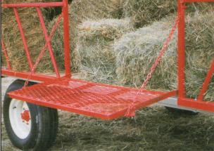
The side doors open to form a horizontal platform, or tilt down 45° for sliding bales into a conveyor.
